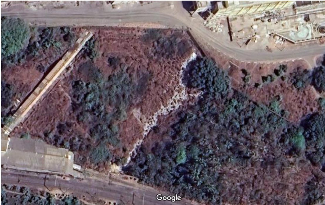
Fig 17: shows Google Earth image of surface runoff traces flowing from the unit
